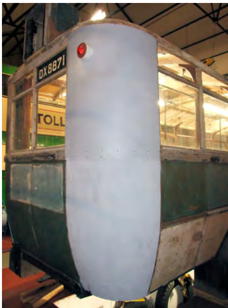
Restoration of Ipswich Ransomes, Sims & Jefferies 44, which dates from 1930, is progressing well. Both rear offside corner panels have been replaced and the rear lamp has been recreated. [Stephen Cobb]
